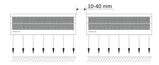
Don't allow gaps between the unit and the wall. When hanging it from the ceiling, using the enclosed ceiling brackets.
